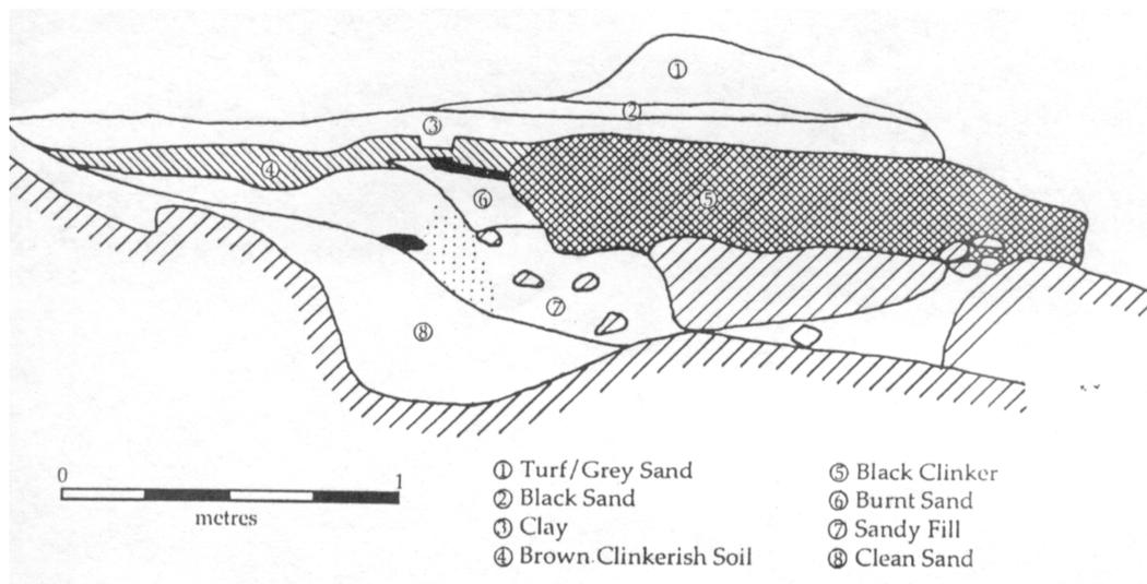
**Figure 15.** Profile Drawing of Wellers Rock Tryworks (Campbell 1993b)
